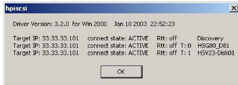
Figure 25: iSCSI Connection Status
